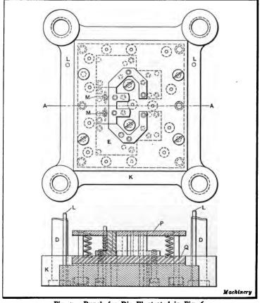
Fig. 7. Punch for Die Illustrated in Fig. 6
